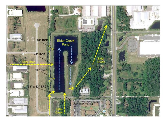
Figure 1-3. Significant Inflows and Water Movement in the Elder Creek Wet Detention Pond.
